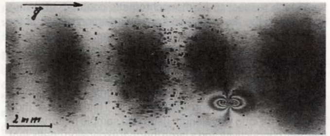
Fig. 6: 0\ 2\ 2 topograph of a silicon-silicon oxide-silicon layer sample ( \lambda = 0.33 \text{ \AA} , E = 38 \text{ keV} )
